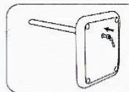
Insert screw and tighten it with ② allen key (Be sure to use ② allen key)
