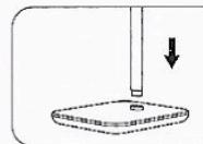
Insert rod fully into base till it clicks into position
